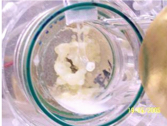
Figure 7: Picture of the casein proteins precipitated on the AFN membrane in the desalination cell during the desalination of milk.
